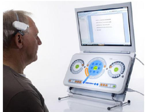
Figure 8. Optical Pointer<sup>(11)</sup>
